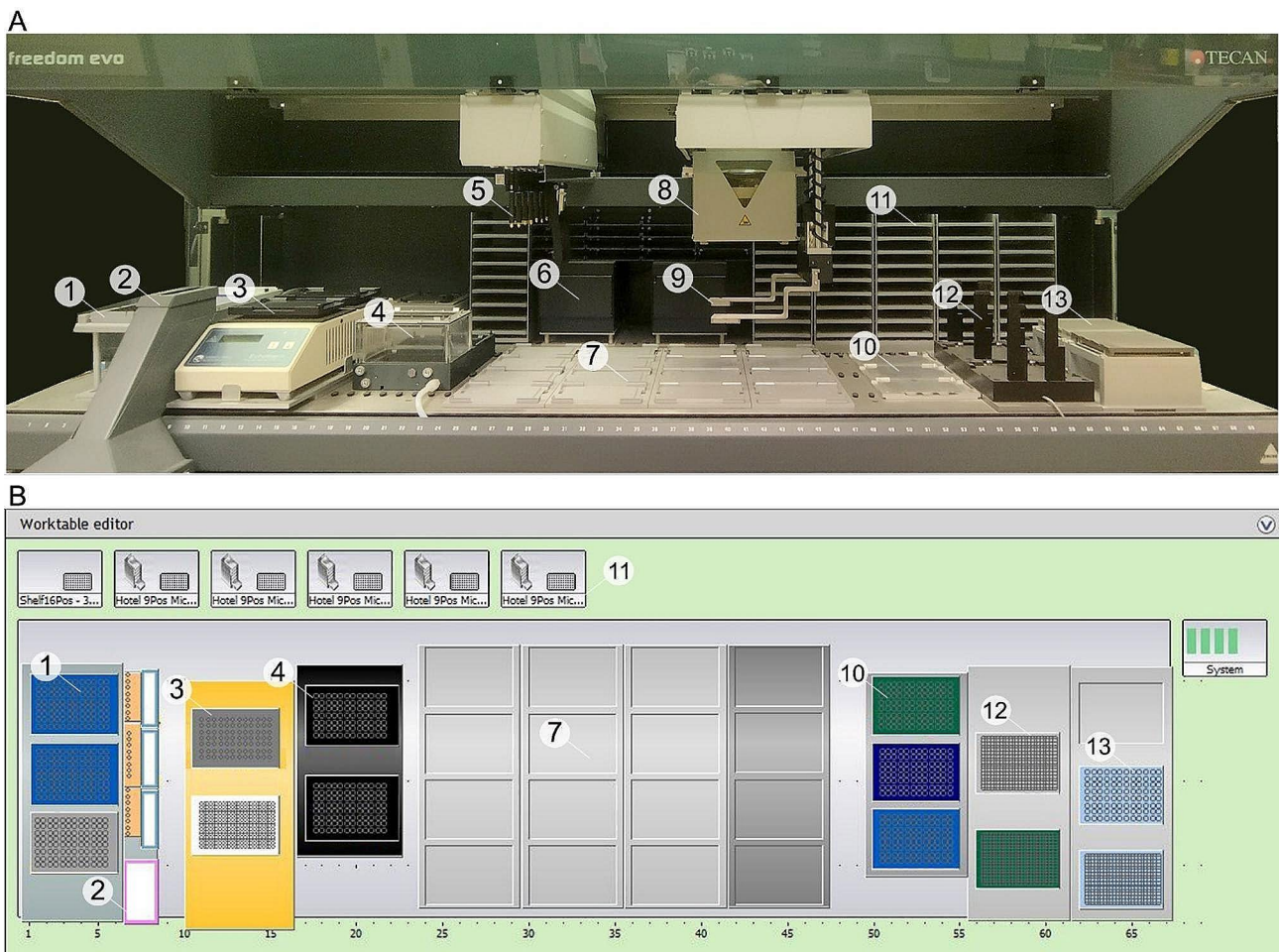
Fig. 2 TECAN Freedom EVO200 system representation. The figure shows the liquid handling platform equipment. (A) Picture of the instrument supplied at the institute’s facility (Stazione Zoologica Anton Dorhn, Naples). (B) Scheme of the workstation. Numbers indicate the main components of the platform both (A) in the picture and/or (B) in the scheme of the workstation: 1, LiHa tips carrier (3 positions); 2, Liquid/Solid waste station (3 plus 1 positions, respectively); 3, Chilling/Heating dry baths (2 positions); 4, Vacuum Separator block (2 positions); 5, Liquid Handling Arm (LiHa); 6, Shaking Heated Incubators (2 positions); 7, Worktable (16 positions); 8, Multi-Channel Arm 96-tip pipetting head (MCA96); 9, Common Gripper Module (CGM); 10, MCA tips carrier (3 positions); 11, Plate Hotel shelf (6 positions); 12, MCA 384 tips support (2 positions); 13, MCA Head adapters
