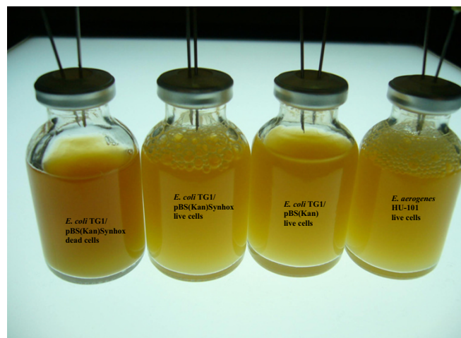
Figure 2 Hydrogen production with E. coli TG1/pBS(Kan)Synhox and E. aerogenes HU-101 (hydrogen bubbles shown). Representative samples shown from hydrogen assay experiments in complex medium with glucose (repeated 3 times).
