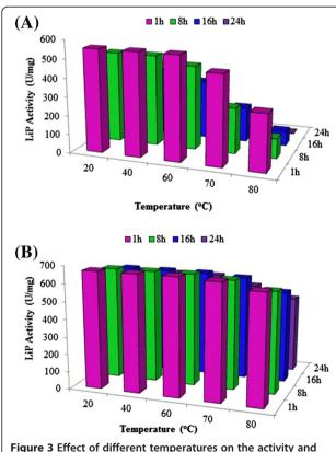
Figure 3 Effect of different temperatures on the activity and stability of purified free (A) and xerogel matrix immobilized (B) *T. versicolor* IBL-04 LiP.
